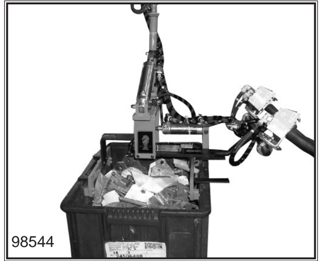
I.D. clamp style fixture to transfer bin
