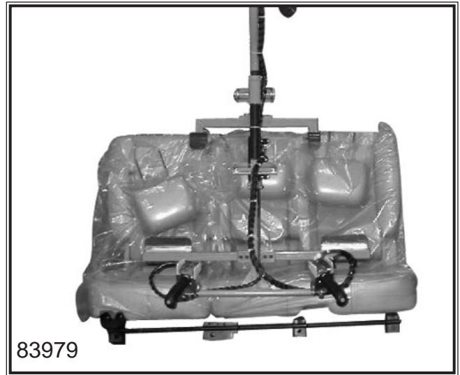
Rear Seat clamping fixture to transfer seats on dunnage
