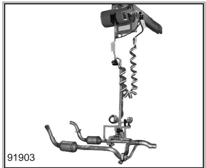
Hook style fixture to install y-pipe with 90° power rotate
