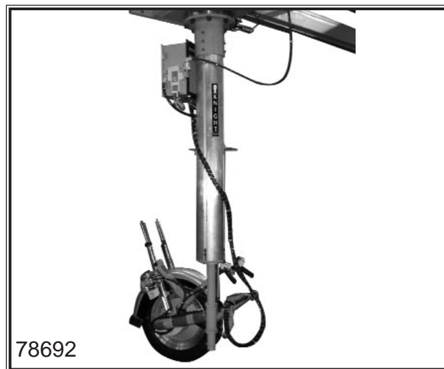
Clamp style fixture to transfer motorcycle front end
