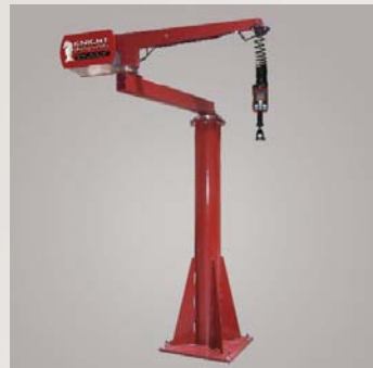
▲ KSHAEA Servo Hoist Articulating Extension Arm "Floor Mounted" Articulating Extension Arm attached to a Servo Hoist. Allows for overhead extended non-linear reach within a work cell. May be mounted to a single bridge, rotating carriage, or floor mounted pedestal.
