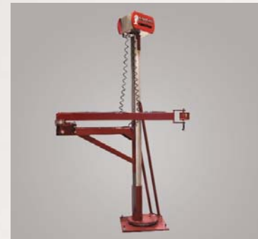
▲ KSHVAA Servo Hoist Vertical Articulating Arm "Floor Mounted" Servo Hoist mounted on a vertical aluminum mast. Creates a steady state condition, eliminating the yarding of the chain. This hoist includes an articulating boom which enables the operator to reach underneath areas in a confined work cell.
