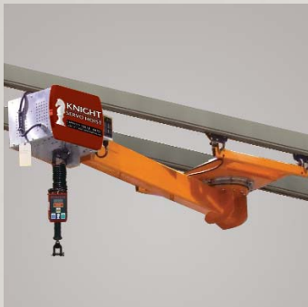
▲ KSHEA Servo Hoist Extension Arm "Overhead Carriage" Servo Hoist attached to an Extension Arm. Allows for overhead extended non-linear reach within a work cell. May be mounted to a rotating carriage or floor mounted pedestal.
