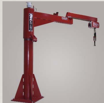
▲ KSHAEA Servo Hoist Articulating Extension Arm "Floor Mounted" Articulating Extension Arm attached to a Servo Hoist. Allows for overhead extended non-linear reach within a work cell. May be mounted to a rotating carriage or floor mounted pedestal.
