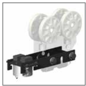
Rail Brake Pneumatic stop that allows operator to park a bridge or arm on the rail. Bolts to most Knight trolleys and end trucks. Model# MRAA4359 (Shown)
