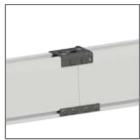
Rail Splice Joins runways or monorails. A hanger must always be used within 12 inches of a splice for support. Model# MRHA7503 (Shown)
