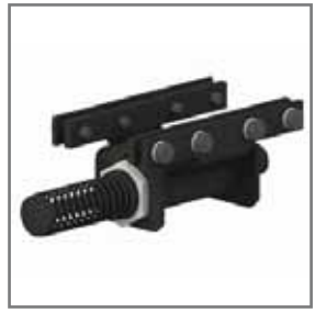
Mid-Rail Stop with Shock Typically used to separate the working area of a bridge or runway and/or to prevent a bridge from over travel. Model# MRAA4498 (Shown)
